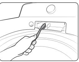
**4.** To clean the drawer opening, use a small, non-metal brush to clean the recess. Remove all residue from the upper and lower parts of the recess.
