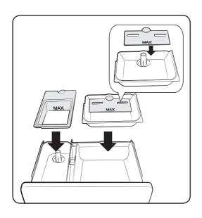
**3.** Remove the inserts from the 3 compartments. Rinse the inserts and the drawer with warm water to remove traces of accumulated laundry products.
