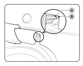
**5.** Return the inserts to the proper compartments and replace the drawer by placing the **dispenser drawer rail (B)** on top of the **compartment rail (A)** (Tilt the dispenser drawer downward and insert it).
