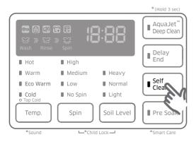
Self Clean is a self-cleaning cycle that removes mold that may occur inside the washer.
