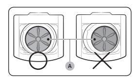
See if the washer is level by checking the position of the tub:
