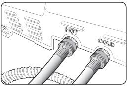
**4.** Connect the ends of the water supply hoses to the water supply intake connections at the back of the washer.
