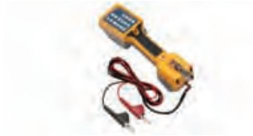
The TS22 test set's unique built-in amplified speaker provides three audio levels for hands-free listening and use with automated voice response systems. The TS22 unit offers a combination of reliability, durability and expanded utility.
