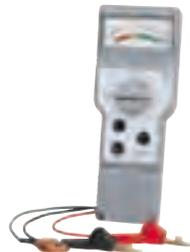
Performs the patented Stress Test which reads audible noise produced on a faulted pair that is stressed by a 90 dBmC excitation. This identifies DC resistive or capacitive imbalances. The patented Leakage Test detects intermittent faults that do not appear under normal VOM tests by using 135 V to "punch through" the oxide layer and reveal a cable fault. The Sidekick Plus includes an RFL and TDR.
