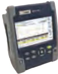
Testing metro, cable TV (CATV), access and fiber-to-the home (FTTH) networks with a larger crew calls for using high-performance handheld test equipment which is both cost-effective and versatile. Whatever your needs, the T-BERD/MTS-2000 can provide an optimized OTDR. The large display combined with a comprehensive user interface makes it the ideal OTDR to respond to any test scenario. The TB2000 provides a rugged, battery-operated handheld test solution.
