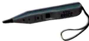
The filter probe blocks AC interference by filtering out power-related noise to stop 60 Hz power line hum. The 200FP features adjustable sensitivity control/volume, a momentary ON/OFF push-button and recessed terminals for connecting the unit to telephone test sets or headphones. Works with most tone generators.
