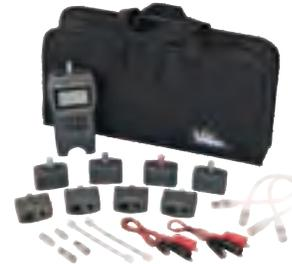
The VDV PRO cable tester is an easy-to-use cable testing and verification device that can quickly test all wiring requirements found throughout today's residential and commercial environments. This tester tests for opens, shorts, split pairs, reversals and miswires on UTP cables, and opens and shorts on coax. It supports RJ11/12, RJ45, coax, F, BNC and RCA connectors. The IENet PRO version supports RJ45 and MJ12 connections and tests to PROFINET industrial Ethernet cabling requirements.
