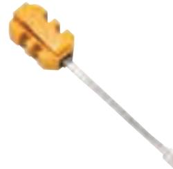
The In-line Modular Adapter permits testing on working lines without disrupting service and helps determine whether the trouble is in the phone or in the line. This unit works like the Fluke Networks standard modular adapter, but has the added feature of replaceable test leads.
