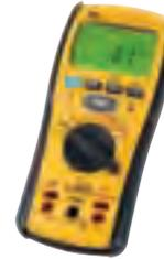
The IDEAL #61-797 digital insulation meter is the tool needed to determine whether the insulation is performing at an effective and safe level. It verifies the integrity of insulation in cables, motors and other devices to keep current flowing safely through the copper conductor. The meter identifies capacitive, absorption and leakage current, helping to prevent problems before they result in injury or equipment failure. This tester is rugged and built for industrial and commercial applications.
