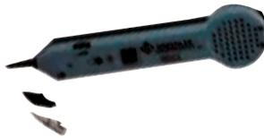
Used in conjunction with any tone generator, inductive amplifiers permit wire and cable identification without having to make direct metallic contact with the conductor. All models feature a powerful speaker for noisy environments, adjustable volume control, recessed on/off button control and high gain for accurate wire identification in congested cable bundles.
