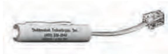
A pencil-sized test device for testing analog telephone lines at the connecting block or network interface. This device will check for open line, polarity, AC voltage and dead line. On digital lines, it may or may not show voltage present.
