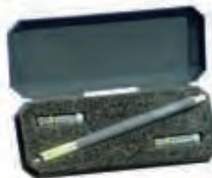
The Corning Cable Systems VFL-350 Visual Fault Locator/Light Source is used to check single-mode and multimode optical fiber cables and components for faults or to locate individual fibers in a bundle. By transmitting a bright beam of red light into a fiber, breaks or improper terminations can be seen as a glowing red light. The VFL-350 emits visible laser light of 635 nm with an output power less than 1 mW. The robust and compact metal housing makes the device suitable for daily on-site use.
