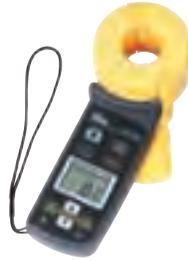
The IDEAL 920 series ground resistance tester enables users to test grounding systems without disconnecting the ground, saving both time and effort. By simply clamping around the grounding rod or ground conductor, it provides direct measurements of both ground resistance and ground leakage current.
