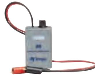
The Model 88 Load Coil Detector is designed for use on telephone cable by outside plant or central office personnel. Allows telephone personnel to quickly and easily indicate the presence and number of load coils (up to four) on an active or dead cable pair. The detector is lightweight and uses one 9 V battery.
