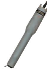
The economical, re-designed VFF5 visual fault finder is a light source used to locate breaks and misconnections in fiber optic cables. A hand-held battery-powered tool, the VFF5 projects highly visible red light into a fiber optic cable. The VFF5 is equipped with a high-power, extra-long-life, 650 nm laser which operates either in continuous (CW) or modulated mode up to 3 km (2.3 miles) into multimode fiber and 4 km (2.5 miles) into single-mode fiber.
