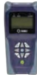
Perform network testing functions including port discovery, PoE test, ping, hub flash, CDP and high-end cable testing including length measurement. Monitor and correct network problems associated with the physical layer and link conditions of the network. Results are displayed in a wiremap format with a pair by pair status message.
