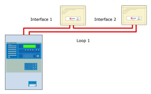
5. Remember the Loop Interfaces can have a maximum of 31 devices allocated to each individual Interface.
