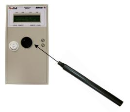
**STEP 6** Present and hold the device survey tool against the wall or ceiling in the position of the proposed installed device.
