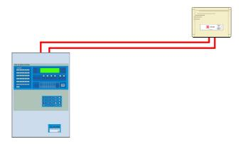
2. Remember to achieve maximum signal range, the Loop Interface should be installed 600mm away from metal objects and other equipment and 2 metres from electrical equipment. This allows free space around the Loop Interface's internal aerials.
