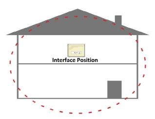
4. Remember when choosing a location the Loop Interfaces require a loop in and out cable connection and a maximum of two interfaces per loop are allowed.
