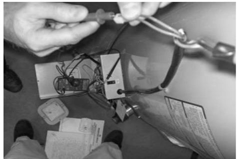
Checking continuity of upper sensor wire harness.
