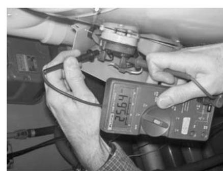
Checking pressure switch contacts. Contacts are open if blower is operating and there is 22-26 volts measured between the two contacts (as in photos)
