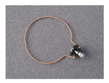
The experiment was successfully repeated with a light bulb 24~V~/~100~W (the whole class can see it). The light bulb 24~V~/~100~W can be purchased in any wholesale shop. For that purpose, we used the coil in diameter 11~cm (a plumber pipe can be used) made of four turns of insulated conductor of  $1mm^2$  size. This coil is connected to the bulb socket.
