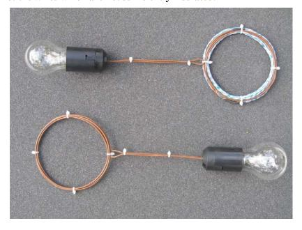
The last experiment was done with the largest easily available light bulb 230 V / 0,5 kW. The same coil as in the previous experiment was used (40 turns), but a larger socket is necessary (equipped by thread E40). To light the bulb, we have to use the pot with the water. After taking the pot away, the bulb remains lit up – the consumption of the bulb is recognized as sufficient to be seen as regular pot on the surface of the plate.
