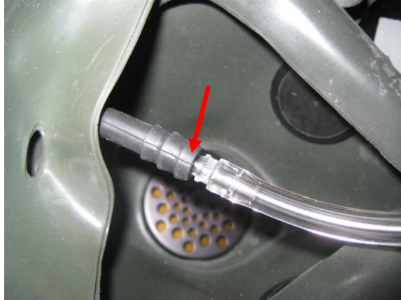
Example of DT Sample Hose installed on internal DT mouthpiece. This configuration may vary depending on the mask being tested.
