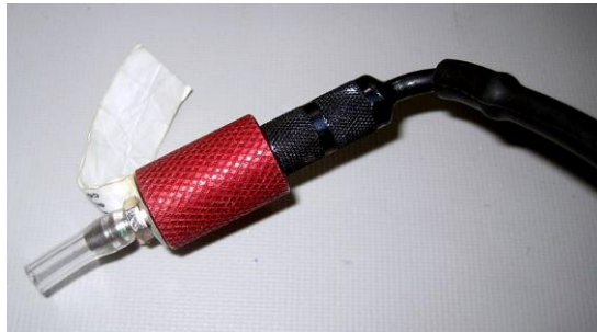
Example of DT Adapter installed on DT Valve. This configuration may vary depending on the mask being tested.
