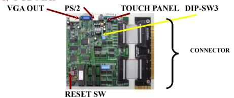
• **Reset SW**: Switch it when power is OFF to clear record. The game setup data will NOT be clear by RESET SW.
