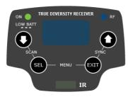
From Status Display push SEL and EXIT together to enter on the Main menu Use UP/DOWN to navigate on all available menus Push SEL to select a menu item Use UP/DOWN to move on the different parameters of the menu Push SEL to modify the parameter menu Use UP/DOWN to change the parameter value Keep push SEL to save changing Push EXIT to return on the Main Menu Push EXIT to return on the Status display
