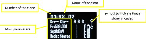
NOTE: the clones are saved on the EPROM and remains saved also after a reboot of the device.
