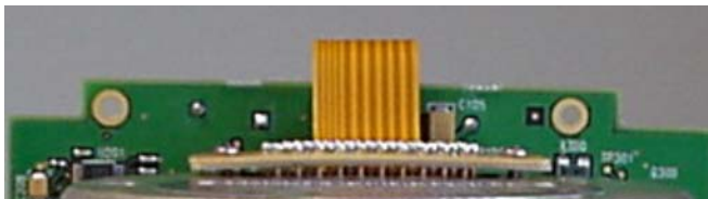
Figure 37: Incorrect (Bowed) Flex Cable Installation
