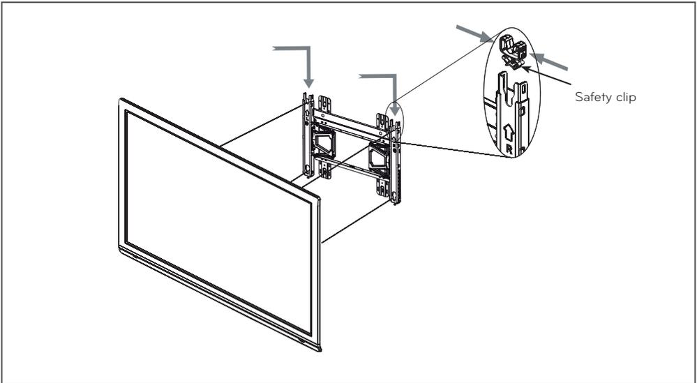
1. Set the display with the guide spacer assembled on the wall mount bracket on the wall in arrow direction. At this time, align the bottom assembly part and lift the set up lightly to align the top part.
