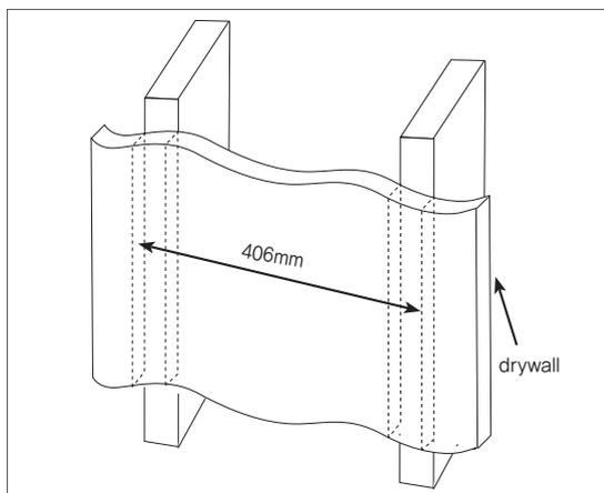
a. Locate and mark the centers of the wall studs using a stud finder.
