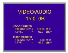
Figure 7.- Video/Audio rate measurement
