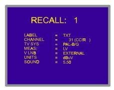
Figure 33.- RECALL screen, retrieving a measurement configuration.
