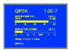
Figure 17.- BER measuring screen for QPSK-modulated signals
