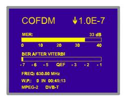
Figure 14.- MER measuring screen for COFDM-modulated signals.
