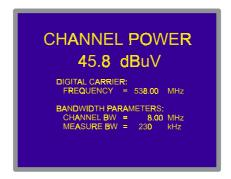
Figure 10.- Digital channel power measurement.
