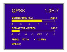
Figure 15.- BER measuring screen for QPSK modulated signals.
