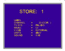
Figure 32.- STORE screen, storing a measuring configuration.
