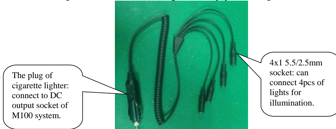
Picture 5: Extension cable 4x1 for DC output
