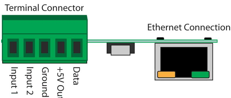
Figure 2.2c - Connector Pinout
