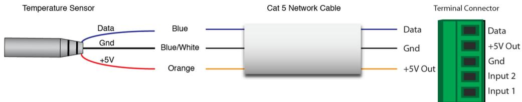
Figure 2.2h - Recommended connection using Cat 5 cable
