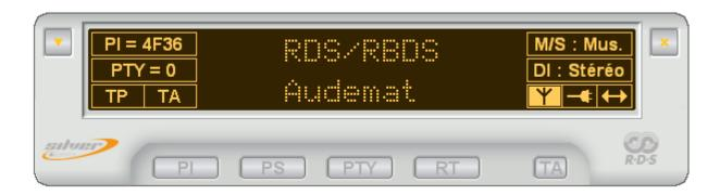
The software has been designed to run with the encoder by means of an RS232C link so as to program it in real time when changing parameter values. It can also save the configurations created in file form: this enables an encoder to be quickly reprogrammed in a given configuration.
