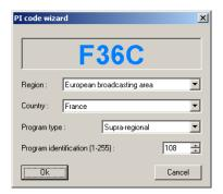
In **RDS** mode, set the various fields (Region, Country, Type of program) and enter the program's digital identifier, then click on **Ok** to confirm: the PI code which is calculated and displayed in the top part of the window will automatically appear in the PI code text zone of the station identification window.
