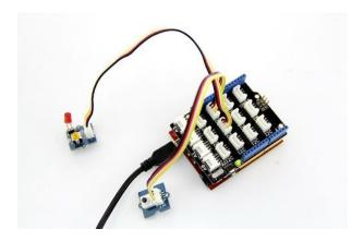
"Momentary" means the button rebounds after pressed . This button output HIGH when pressed, and LOW when released.
