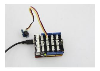
This is an alternative to the momentary button .Grove – Touch Sensor detects the change in capacitance in the circular region; the closer you finger is to the region, the larger the change in capacitance. Even if there is paper between your finger and the sensor, it will still function reliable.
