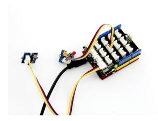
The output of the analog light sensor ranges from 0 to 1023, but the output is not linear with respect to the ambient light intensity.
