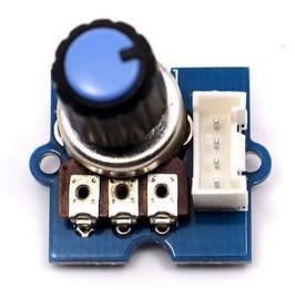
The potentiometer Grove produces analog output between 0 and VCC. The angular range is 300 degrees with a linear change in value. The resistance value is 10k ohms, perfect for Arduino use.
