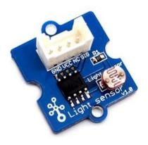
The light sensor, also known as the light dependent resistor (LDR). Typically, the resistance of the light sensor will decrease when the ambient light intensity increases.
