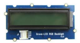
This Grove enables you to set the color to whatever you like via the simple and concise Grove interface. It takes I2C as communication method with your microcontroller. So number of pins required for data exchange and backlight control shrinks from ~10 to 2, relieving IOs for other challenging tasks. Besides, Grove - LCD RGB Backlight supports user-defined characters.
