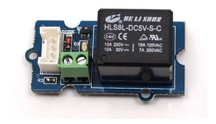
Relay is a useful tool to magnify your Arduino's control ability! Feed the control signal through the Grove interface, and relay will control the open/close of the external circuit that connected to the screw terminals. The voltage of the external circuit can run up to 220V! So grab this relay and start some really tough projects!
