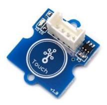
Grove - Touch Sensor enables you to replace press with touch. It can detect the change in capacitance when a finger is nearby. That means no matter your finger directly touches the pad or just stays close to the pad, Grove - Touch Sensor would outputs HIGH.
