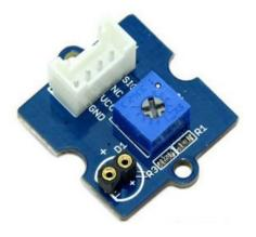
Grove - LED is designed for the beginners of Arduino/Seeeduino to monitor controls from digital ports. It can be mounted to the surface of your box or desk easily and used as pilot lamp for power or signal.
