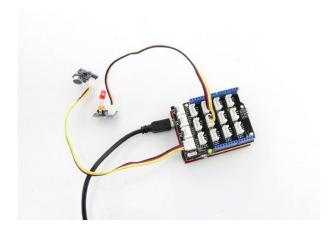
The electric microphone collects sound intensity for all frequencies. And the potentiometer acts as the doorman. When you rotate it completely clockwise, it lets everything go through, and when you rotate it completely counterclockwise, none of it can go through.
