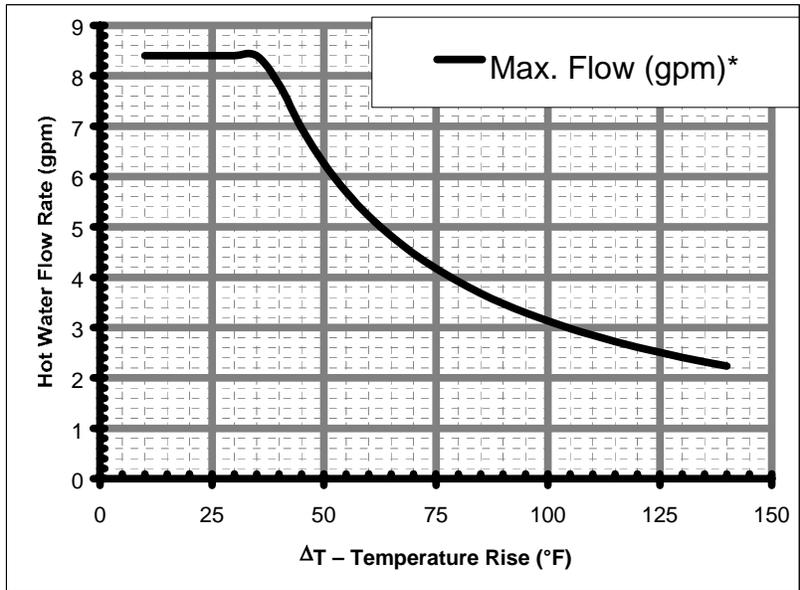
**\*Note: The maximum flow is based upon a minimum water pressure of 30 PSI**
