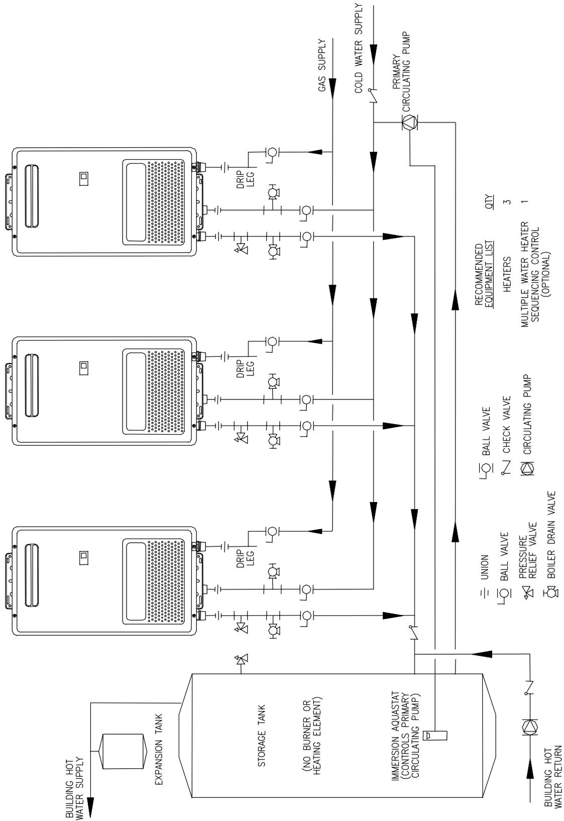
**Note: The Primary Circulator for the water heating loop must be sized for 21 GPM @ 35 Ft. Head**
