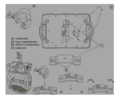
Screw the half cheeseboro or "C" clamp (not provided with the fixture) onto the U bracket supplied with **Elektralite LED Pro Line Pancake.**
