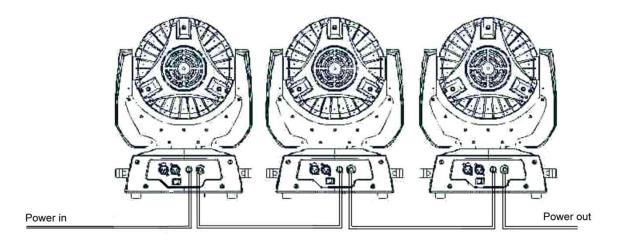
There can be up to 7 **Elektralite LED Pro Line Pancake** in the daisy chained line. The line is fused protection against more than this quantity being daisy chained. So do <u>NOT</u> exceed this number of fixtures.
