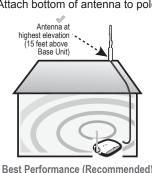
Place External Antenna on roof or in attic
