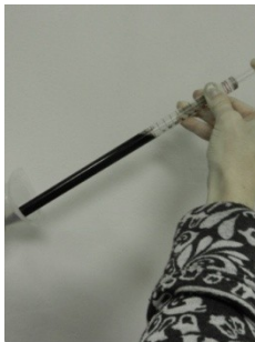
Figure 5. Dispense 25 mL of your wine into the titration beaker using the 25 mL sampling pipette. Make sure this is clean before putting the pipette into your wine container!
