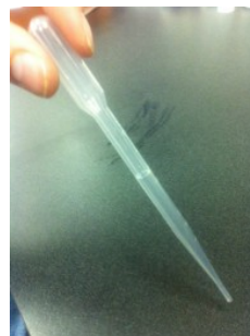
Figure 6. The transfer pipette. One full squeeze of the transfer pipette in either the Acid solution or Reactant should be
