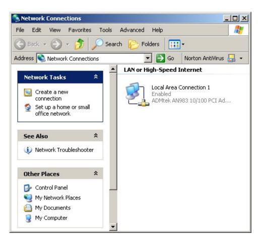
2. Locate the Local Area Connection icon that resembles your Ethernet device. The name of your ethernet device will be printed just below "Local Area Connection". In this example the ethernet device is a ADMtek AN983 10/100 PCI adapter. Use the RIGHT mouse button and click the Ethernet device. A sub-menu will appear. Use the LEFT button and click Properties. The properties for your Ethernet device will appear.
