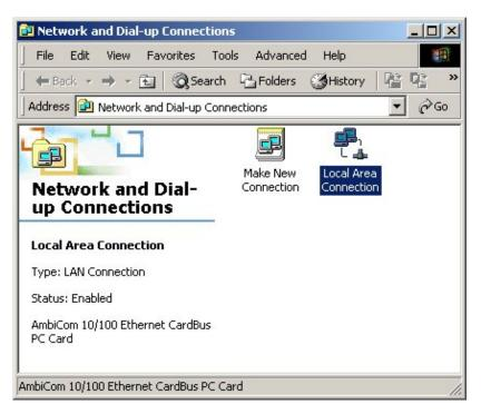
Locate the Local Area Connection icon for your Ethernet device. When you highlight the icon you can see a description of the icon in the left frame as pictured above. In this instance the Ethernet device was a AmbiCom 10/100 Ethernet CardBus PC Card.
