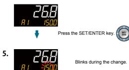
$\Delta \nabla$  Change the setpoint using the Up/Down arrow keys to  $\overline{\triangleleft}$   $\triangleright$  increase and decrease the value and the Left/Right arrow keys to move between digits.
