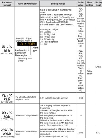
For the alarm function setting parameter, 8 alarms are displayed for the factory default. The number of alarms can be changed by the setup parameter ALNO. (number of alarms). To change the number of alarms, see User's Manual.
