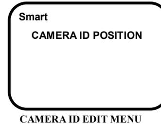
Press UP or DOWN key to select ID POSITION L-U,R-D,L-D or R-U. Then the ID will directly display on the position that you select.
