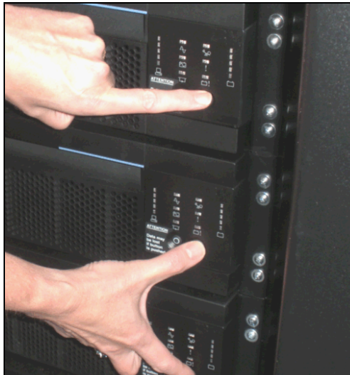
Figure 3-23 Use both hands to hit the three Test buttons simultaneously
