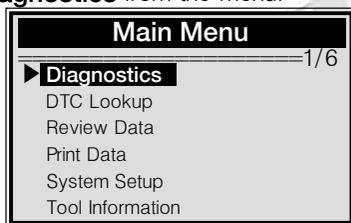
6. Press **ENTER** button to confirm. A sequence of messages displaying the OBD2 protocols will be observed on the display until the vehicle protocol is detected.
