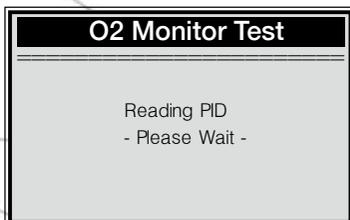
3). Use **UP/DOWN** scroll button to select O2 sensor from **O2 Monitor Test menu** and press **ENTER** button.
