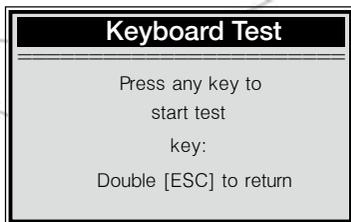
If you press and hold the power switch, the key name does not show on the screen, but resets the scanner when powered by vehicle battery, or turns off the scanner when powered by cell battery. If it does not restart the scanner or power off the scanner, the key is not working properly.
