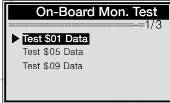
If the vehicle under test does not support the mode, an advisory message will be displayed on the screen.
