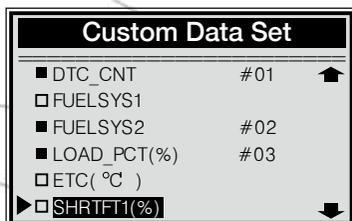
You are allowed to pick up a maximum of 18 PIDs. If the selected PIDs exceed 18, a **"The selected data list is full!"** message displays on the screen.
