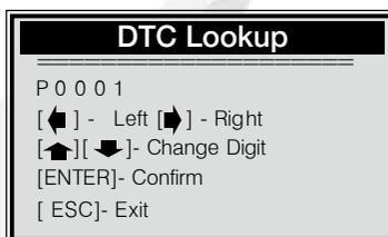
3). View the DTC definition on screen. When DTC definition covers more than one screen, use **LEFT/RIGHT** button to view additional information on previous/next screens.
