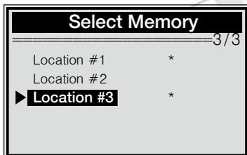
If there is no recording in selected location, a message **"Not Supported or Stored No Data"** displays on the screen.
