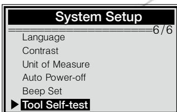
2). Select **Display Test** from **Tool Self-test** menu and press **ENTER** button.
