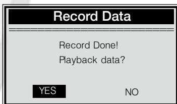
If you wish to playback recorded data, press **ENTER** button; if you do not wish to playback, press **ESC** button, or use **LEFT/RIGHT** button to select **NO** and press **ENTER** button to return to **Record Data** menu.
