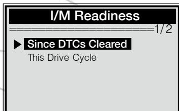
4). Use **UP/DOWN** scroll button, as necessary, to view the status of the MIL light ("**ON**" or "**OFF**") and the following monitors:
