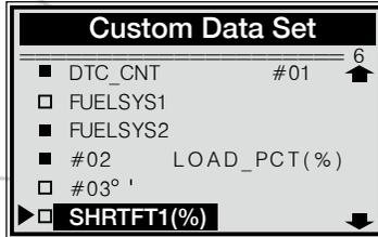
The number "x" to the upper right corner of the screen indicates sequence of highlighted item; and "#x" are the order that the parameters are selected and will be displayed.
