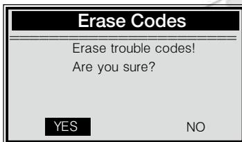
● If you do not want to proceed with erasing codes, press **ESC** button or use **LEFT/RIGHT** scroll button to select **NO** to exit. A message of **"Command Cancelled!"** show ups. Wait a few seconds or press any key to return to **Diagnostic Menu**.
