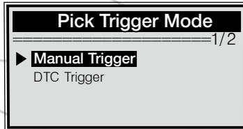
If data from previously tested vehicle is not erased, data from current test will be stored in a temporary cache. Following screen shows when **Manual Trigger** is selected:
