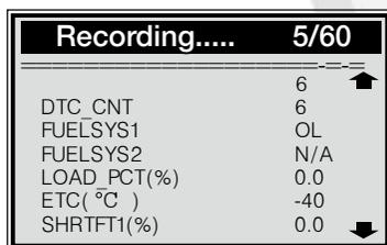
The number "x/x..." to the upper right corner of the screen indicates the maximum frames that can be recorded and the number of recorded frames.
