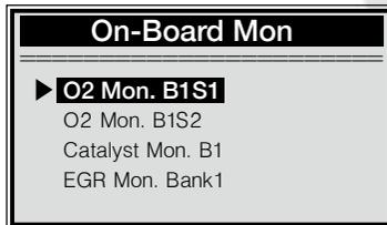
4). Use **UP/DOWN** scroll button to select the desired monitor from **On-Board Mon.** Test menu and press **ENTER** button.
