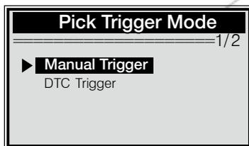
If data from previously tested vehicle is not erased, data from current test will be stored in temporary cache. Following screen shows when **Manual Trigger** is selected:
