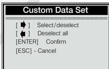
10). Use **RIGHT** button select/deselect data parameters. Selected parameters are marked with solid squares. Press **ENTER** button to confirm.
