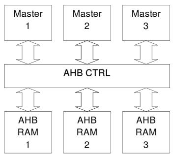
The RAMs must still be 1 MB wide. They must be connected to the three different addresses:
