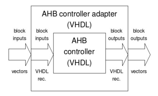
The most internal entity is the AHB controller itself provided by Gaisler research. The AHB controller adapter is a VHDL entity which converts the VHDL records inputs/outputs of the AHB controller into VHDL vectors. These outputs can be interfaced with a Verilog environment because the inputs and outputs of the blocks are vectors and not records.
