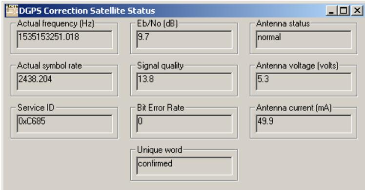
Figure 5 DGPS correction satellite status window
