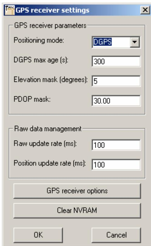
Figure 13 GPS receiver settings window
