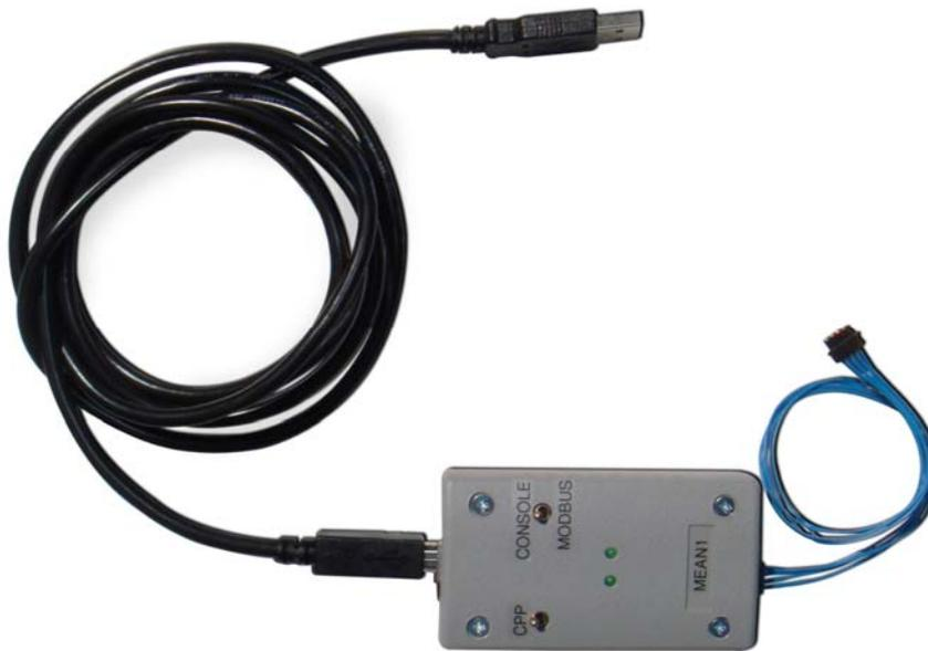
**Photograph 3 USB to Console port interface type MEAN1**
