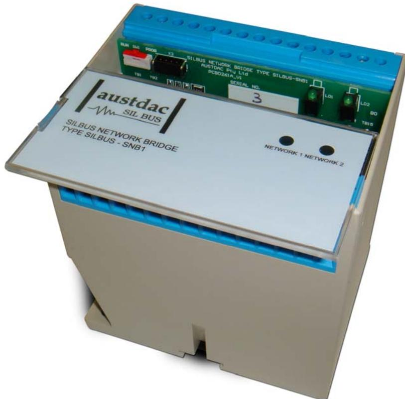
Photograph 2 Access to console ports and programming switches
