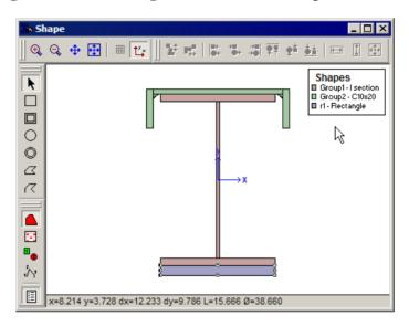
> Release the mouse button when the plate is the correct size, i.e. when the coordinates read x=4, y=-6.5
