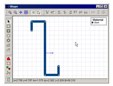
If you have the Grid turned on then the vertices of the polygon will align to the grid. The new shape will be immediately added to the list of shapes displayed in the Data window.
