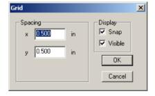
If you want to have the shapes automatically align with the grid but don't want to see the grid, simply click on the Invisible button before clicking OK. Similarly you can click on the Visible button to have the grid displayed as a visual guide but click on the Off button to disable the automatic alignment with the grid.
