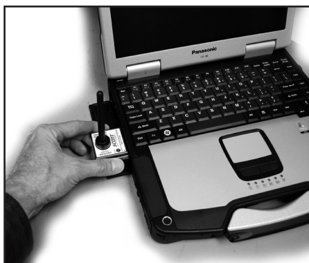
FIGURE 1 INSTALLATION OF THE SEMS II PCMCIA CARD IN A LAPTOP COMPUTER
