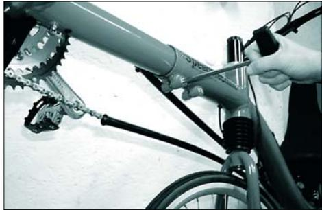
*Unscrew the clamping screws to adjust the front boom.*
