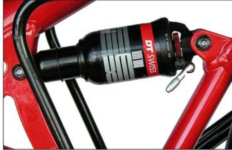
*Air Shock DT-Swiss XM180 Damping ist adjusted with the red knob at the rear end. The shock must be installed with the lock-out lever facing down to avoid a collision of lever and frame when the suspension is moving.*
