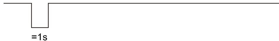
Figure 3-9 The signal through the RING after the MG323 receives an SM
