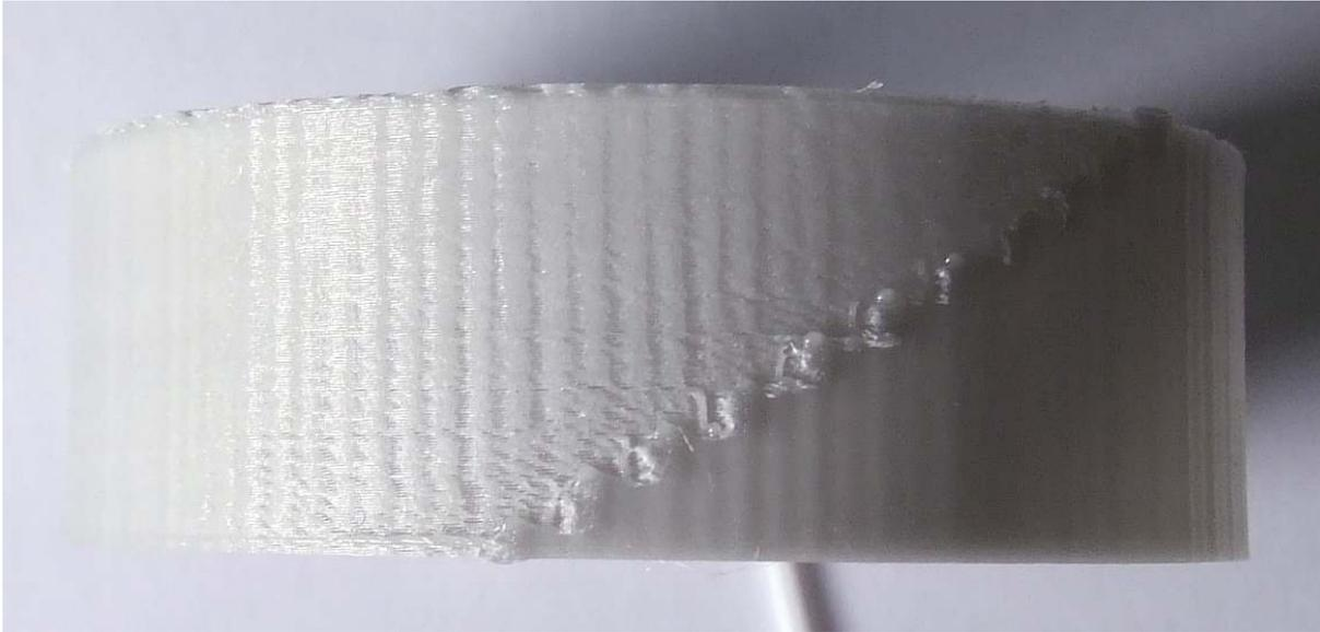
On this picture you can see the low material and too big of retract, material is not properly set back on nozzle after retract.
