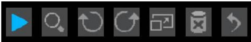
(Pause)    (Zoom out)    (Rotate left 90°)    (Rotate right 90°)    (Ratio)    (Delete)    (Exit)
