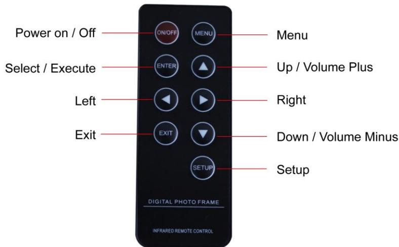
**Note: a)** To edit or adjust, press **MENU** on the remote control; or you can instead press button **Menu** on the frame for 3 seconds.
