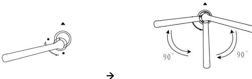
**Note:** Insert the jack of stand into DPF. And then rotate stand 90° to lock the stand.
