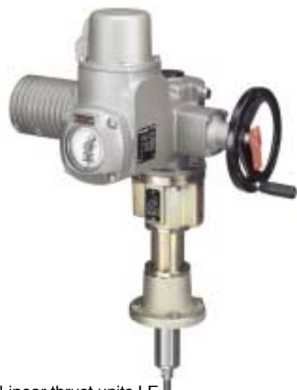
Linear thrust units LE with multi-turn actuators SA Thrusts from 4 kN to 217 kN Strokes up to 500 mm Linear speeds from 20 to 360 mm/min
