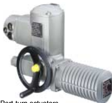
Part-turn actuators SG 05.1 – SG 12.1 Torques from 100 to 1 200 Nm Operating times for 90° from 4 to 180 s
