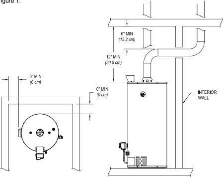
Figure 1. Minimum Clearances for an Alcove Installation.
