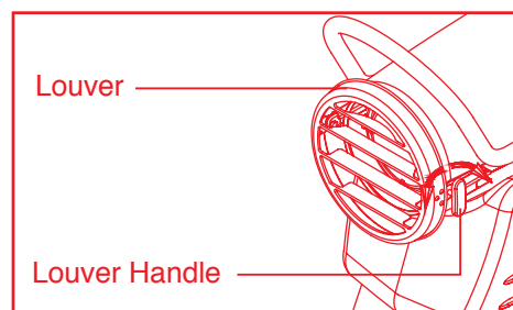
Figure 11. Louver Angle Control
