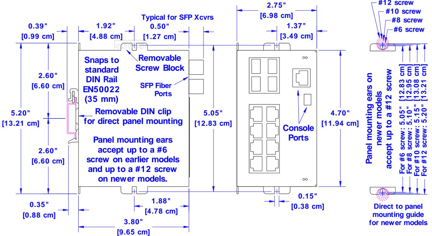
**Mechanical Dimensions for SL/SLX-8MG with 8 Gigabit Ports**
