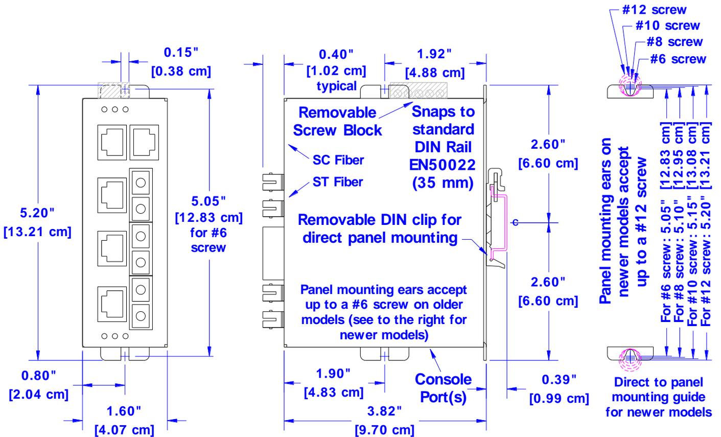
**Mechanical Dimensions for SL/SLX-8ES-6/7 with 3 Fiber Ports**
