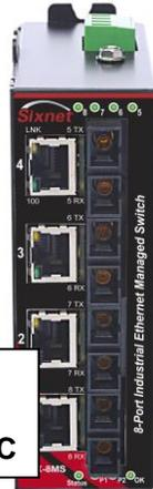
**Typical Fiber Ports on an SL-8MG**
