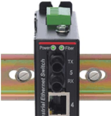
**Vertical screw-to-panel mounting for better shock and vibration resistance.**
