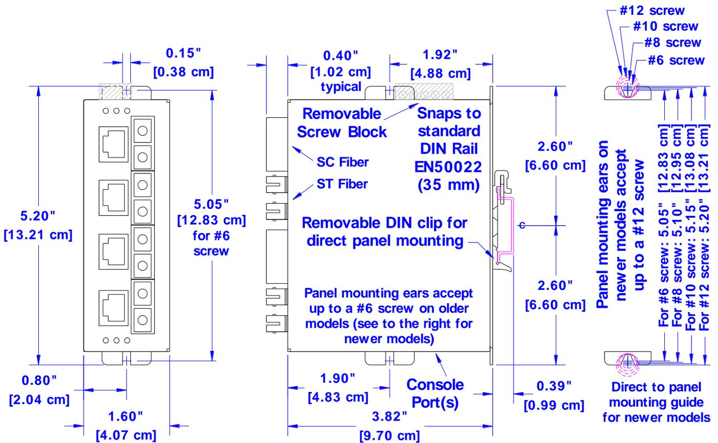
**Mechanical Dimensions for SL/SLX-8MS-8/9 with 4 Fiber Ports**
