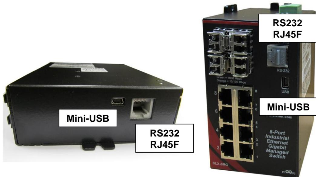
**The RS232 and/or USB ports may located on the bottom edge or front face of the switch**
