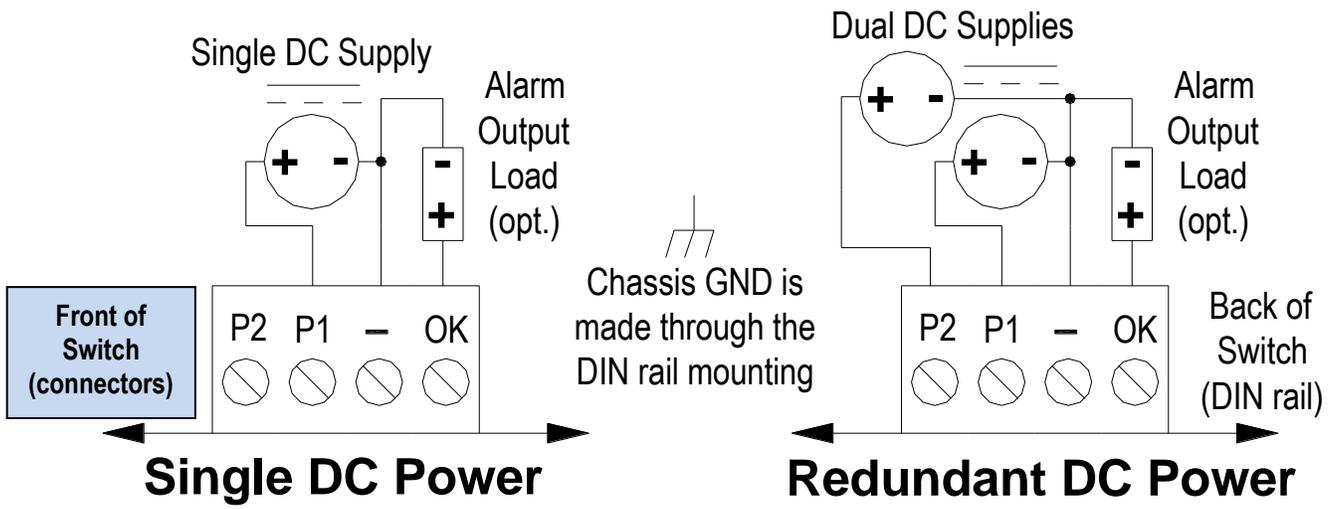
**Power and Alarm Wiring For
