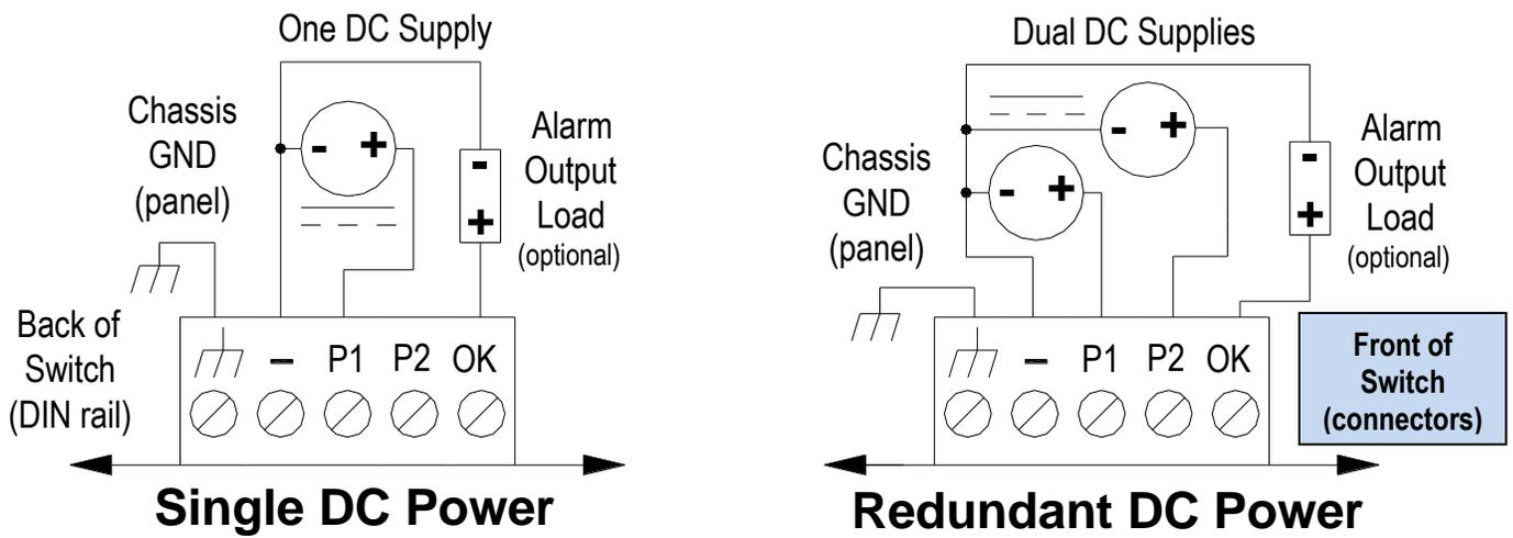
**Power & Alarm Wiring for
