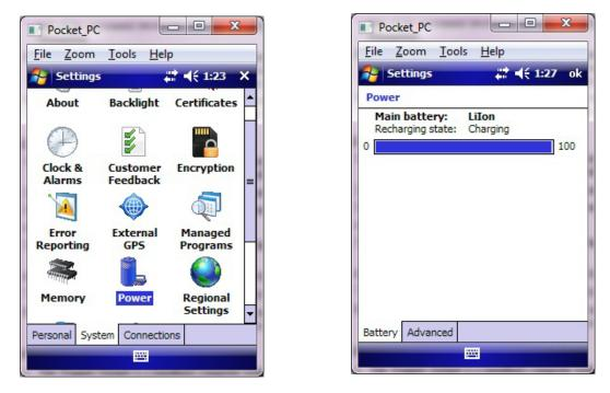
Note that allowing the batteries to become completely drained will erase all settings from the PDA, and may require that the Gadget software be reinstalled. If the batteries in your unit become discharged, you should coordinate with your supervisor to set the Gadget up for field use again.
