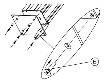
b. FIX COLUMN ASSEMBLY TO WALL
