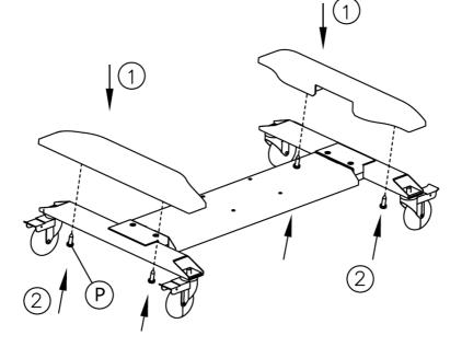
c. ATTACH ASSEMBLY TO COLUMN
