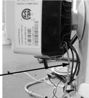
Step 7. Pivot the tool towards the water heater, as far as possible. Lift straight up on the gas control. The gas control should move about 1/8". Hold the gas control in position and remove the tool. Lift straight up on the gas control to remove it completely from the thermal well.
