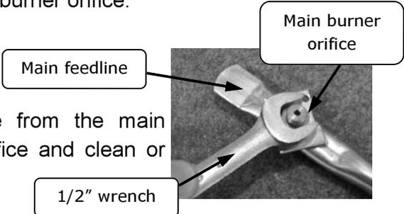
Step 11. Remove the main burner orifice from the main feedline using a 1/2" wrench. Inspect the orifice and clean or replace, if necessary.
