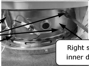
Step 6. Disconnect the pilot tube using a 7/16" wrench and the main burner feedline with a 3/4" wrench from the gas control.
