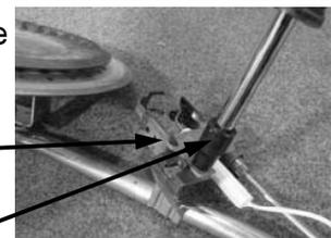
Step 10. Visually inspect the spark igniter/flame sense wire for damage. Replace the pilot assembly, if damage is found.
