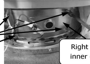
Step 5. Remove (2) 1/4" drive screws from the left side inner door.
