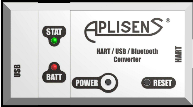
Fig. 1. Front view of the converter.
