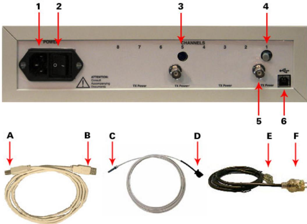
Figure 1 - Opti-Amp Connectors and Cables
