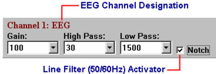
Figure 4 - EEG Channel Layout
