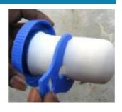
With the plastic sensor you can measure when your filter has to be replaced. When the plastic sensor fits around the thinnest part of the filter, the filter is no longer safe to filter the water and it has to be replaced. Ask your local supplier for the replacement filter.
