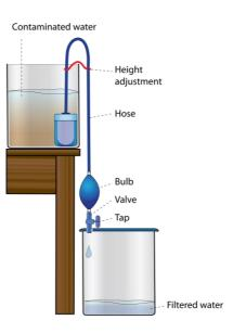
The speed of filtration is faster when the container with contaminated water stands at a higher level.
