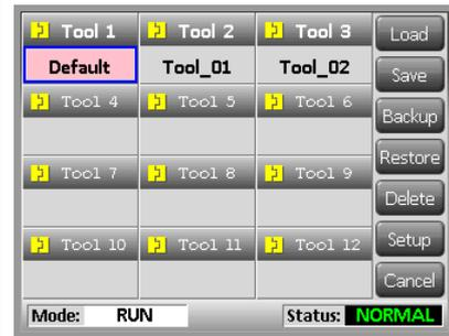
Touch **[Setup]** and enter system password to go to tool configure options
