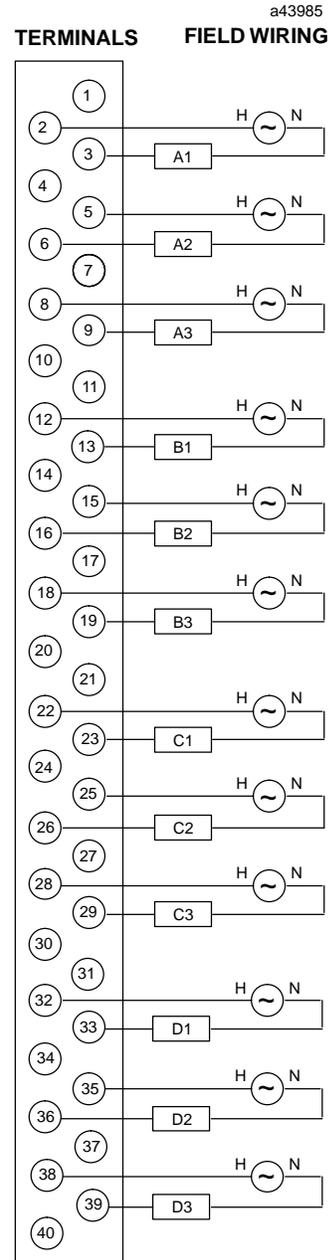
Figure 2. Field Wiring Connections
