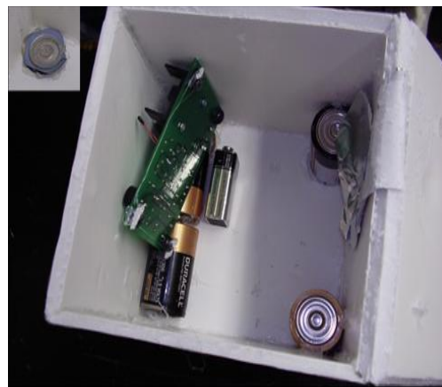
Figure 11.1.E What happened on the inside. The glue did not hold well and we actually ripped a battery bottom off on upper left picture.
