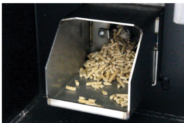
Fuel being delivered into burner
