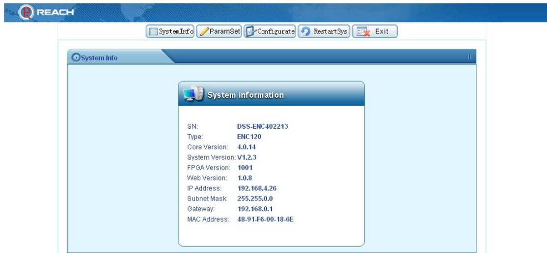
The encoder system configuration interface mainly includes: **system information, parameter setting, system setting, restart and exit.**
