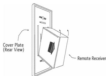
Position the receiver as shown in diagram to the left with lower tab on cover plate inserted into groove of receiver (Make sure ADJ hole and LEARN hole on cover plate properly aligns with remote receiver). Pull receiver up and snap into top tab of cover plate.
