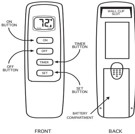
The transmitter operates on (2) 1.5V AAA batteries. It is recommended that ALKALINE batteries always be used for this product. **Be sure the batteries are installed with the (+) and (-) ends facing the correct direction, and are fully charged.**
