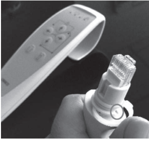
Step 1: Mount the cable lock and fix it to the slot marked in the picture.
